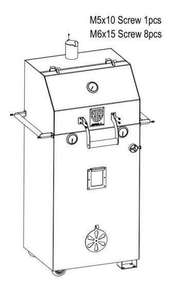
**Step 4: Assemble rotating wheel**Use 2pcs of M5 X 10 Screw to assemble the rotating wheel onto the grill body
